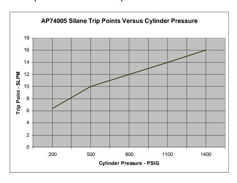
This situation can be avoided by installing the EFS downstream of the pressure regulator as discussed in the next example. In the case of liquefied gases where the cylinder pressure remains constant while the gas is consumed, the trip point will stay consistent if installed between the gas cylinder and the pressure regulator.
