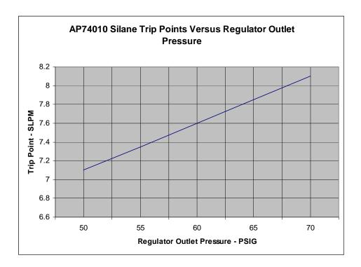
As demonstrated by the graph above, the trip point of the EFS rises only 14% when installed downstream of the regulator in comparison to nearly 200% if the EFS is installed before the pressure regulator.
