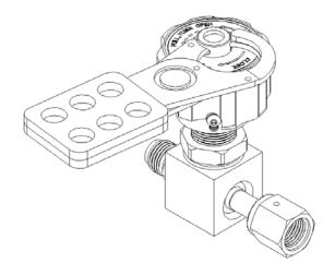
In addition to the passive lock, provisions for a physical lock included. The top of the knob has a swivel hub that enables one to attach 1/8 inch shackle extended length pad lock or a lock hasp such as the Master Lock® # 420. The hub has a cross drilled hole that allows one to insert a leg of the lock or
