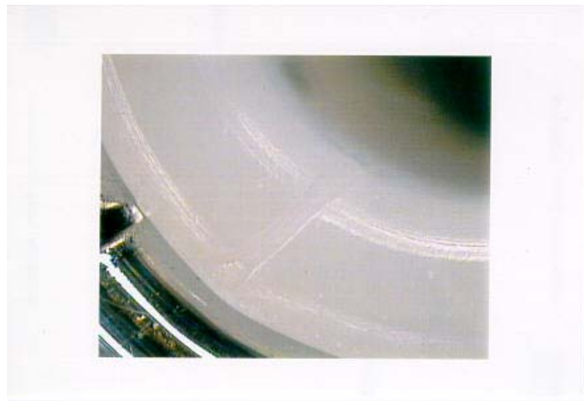
Figure 8. PFA seat after Test #P3 (wire used to create across-the-seat leak) (30X magnification)
