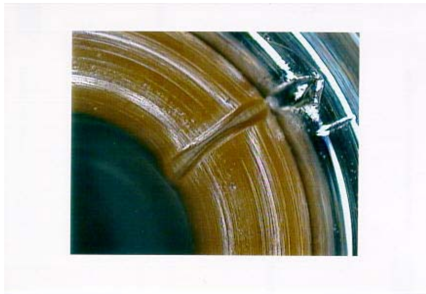
Figure 4. Vespel seat after Test #V5 (wire used to create across-the-seat leak) (25X magnification)
