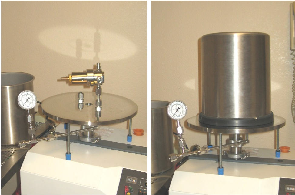
Figure 1. Regulator Across-the-seat Leak Test in Bell Jar
